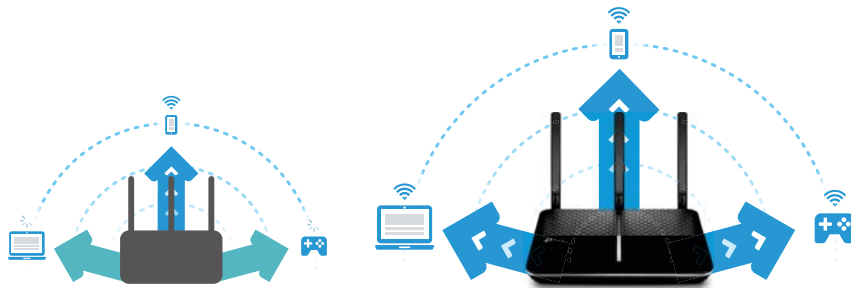
Traditional Router Sends data to one device at a time
