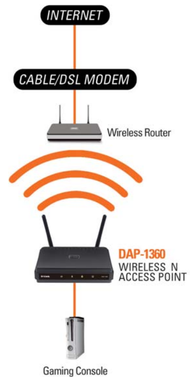
Ethernet-enabled gaming console using the DAP-1360 as a wireless interface to access the Internet
